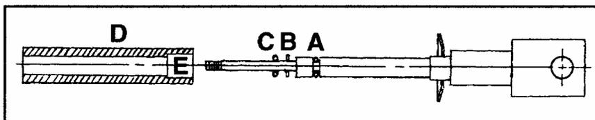
3. Examine sleeves for scoring or etching and replace. **Immerse sleeves (D) in oil and carefully twist and push sleeve onto rod with machined counter bore end first (E).**
