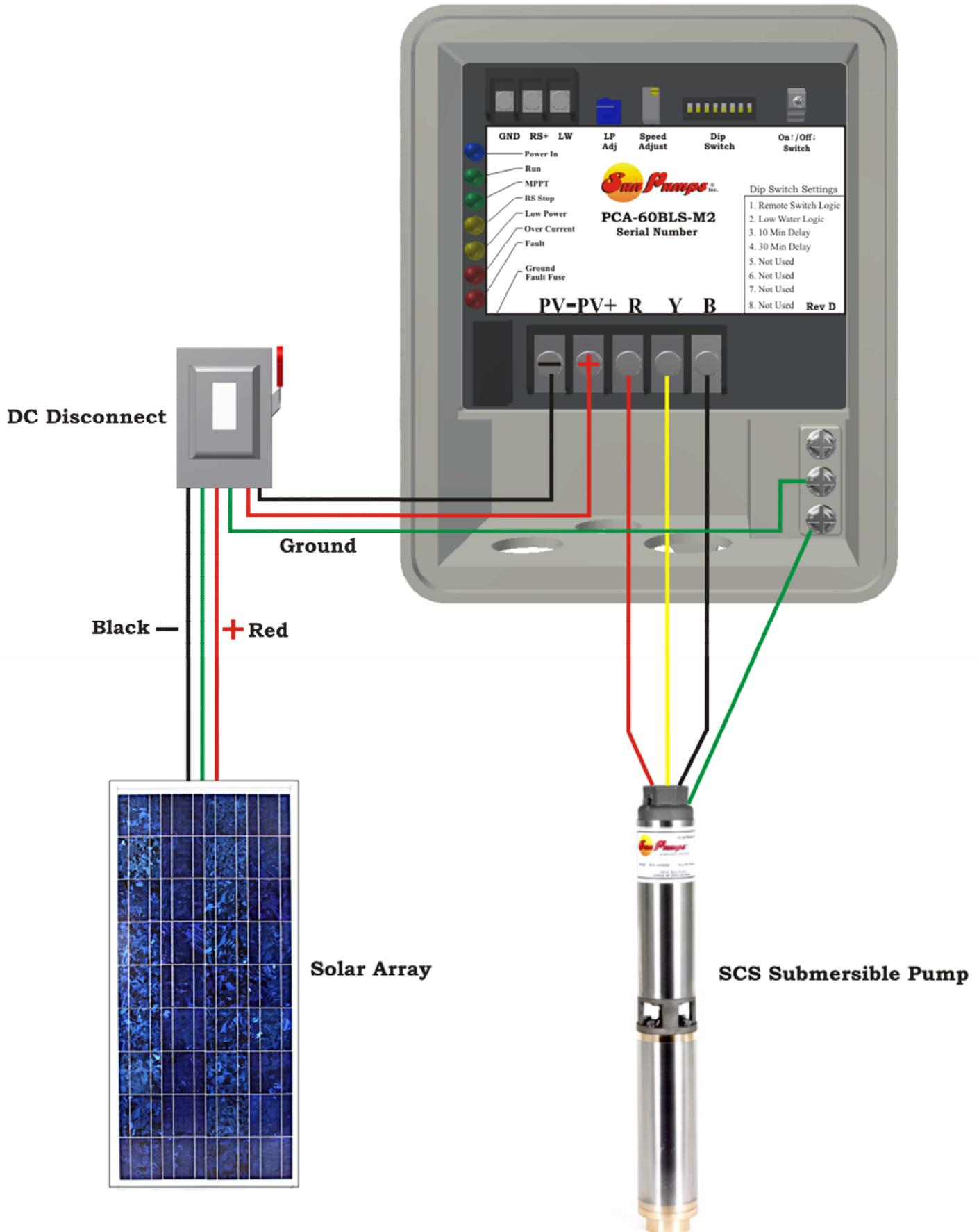
1. Switch the controller to the OFF position.
