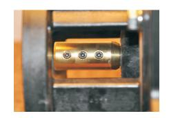
7. Rotate the motor shaft until the key way is at the same 45 degree angle to align with the pump coupling set screws. Apply a small amount of never seize or grease to the motor shaft before inserting into coupling.
