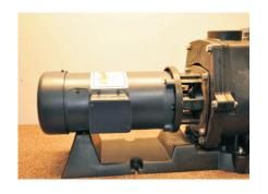
10. Install the four 3/8-16 motor bolts through the motor adapter into the motor and tighten.
