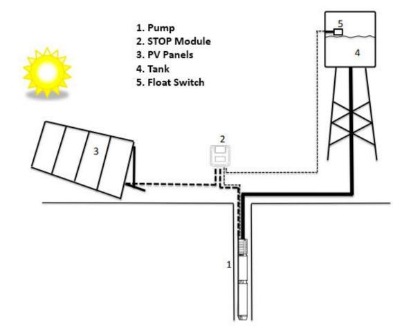
HR DC pumps are equipped, in their standard configuration, with 8 feet flat cable length.
