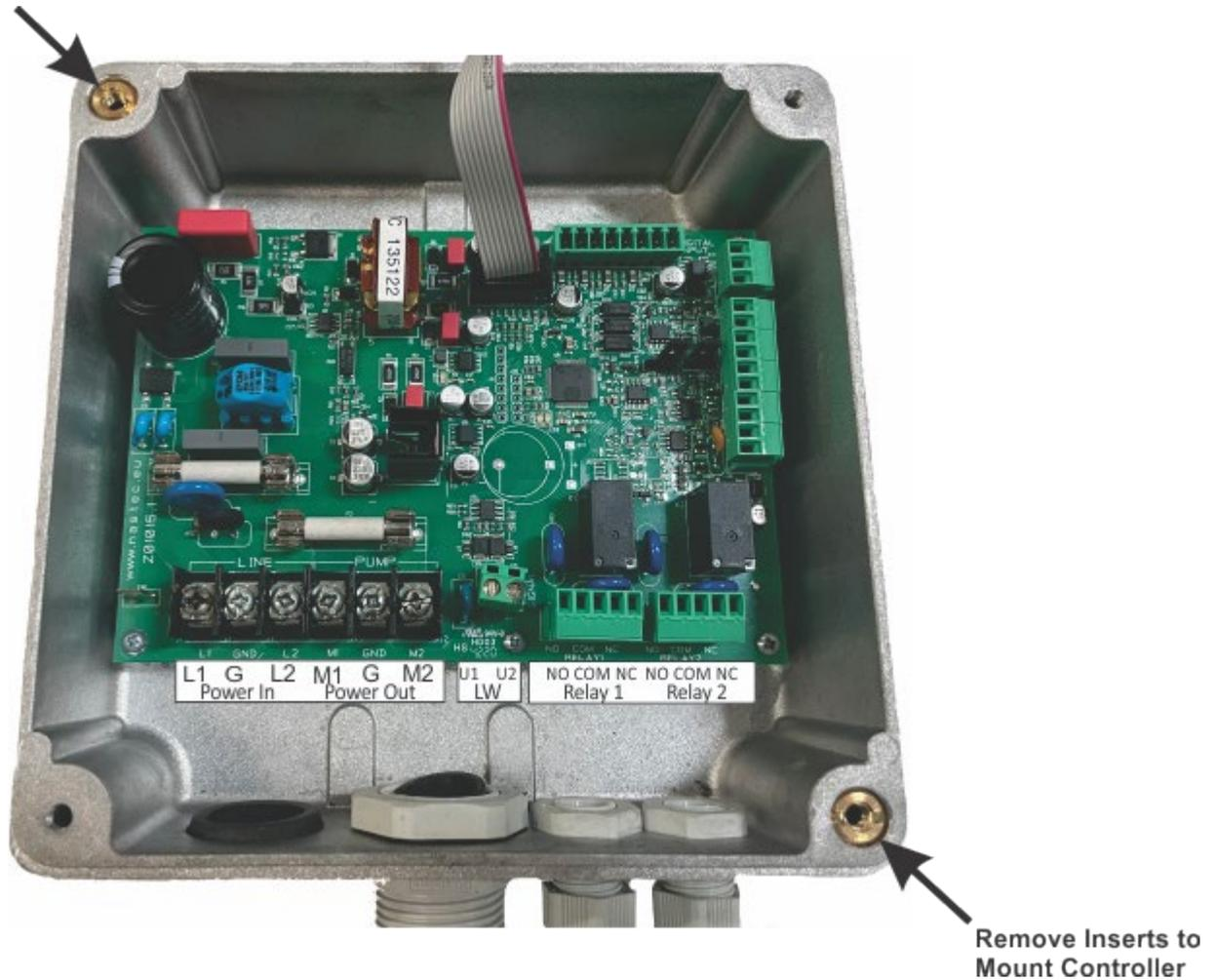
Then, replace the special inserts so the cover can be attached.
